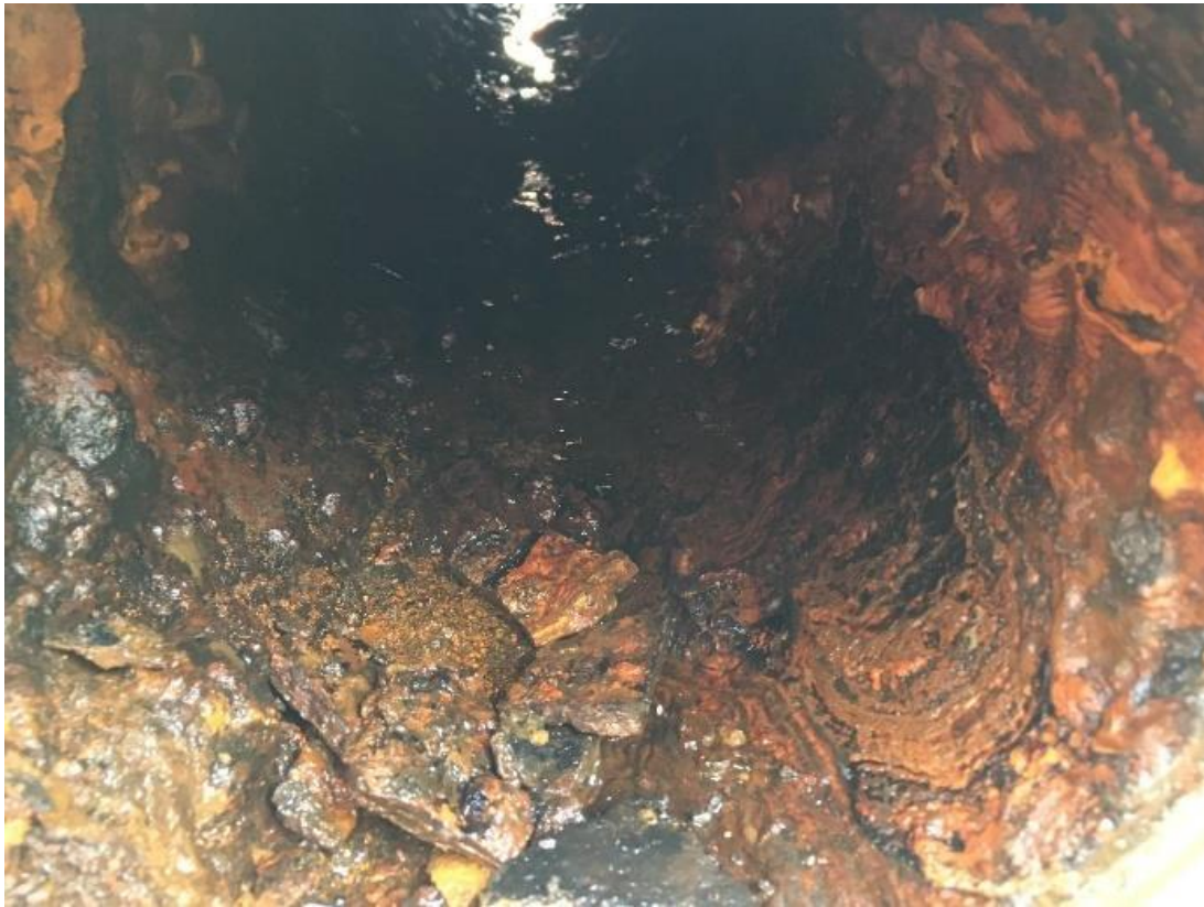
Fig 3 Original pipe, in poor condition as taken out of service
